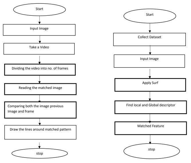
Fig 4:Flowchart of step followed In image processing Fig 3:Flowchart of step followed In Video processing
